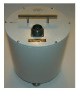
The SP-400-U instrument is designed as a versatile, very rugged medium period seismic sensor. Unlike traditional seismometers, they are based on proprietary electrochemical transducer technology. These instruments have many advantages over conventional electromechanical sensors.
